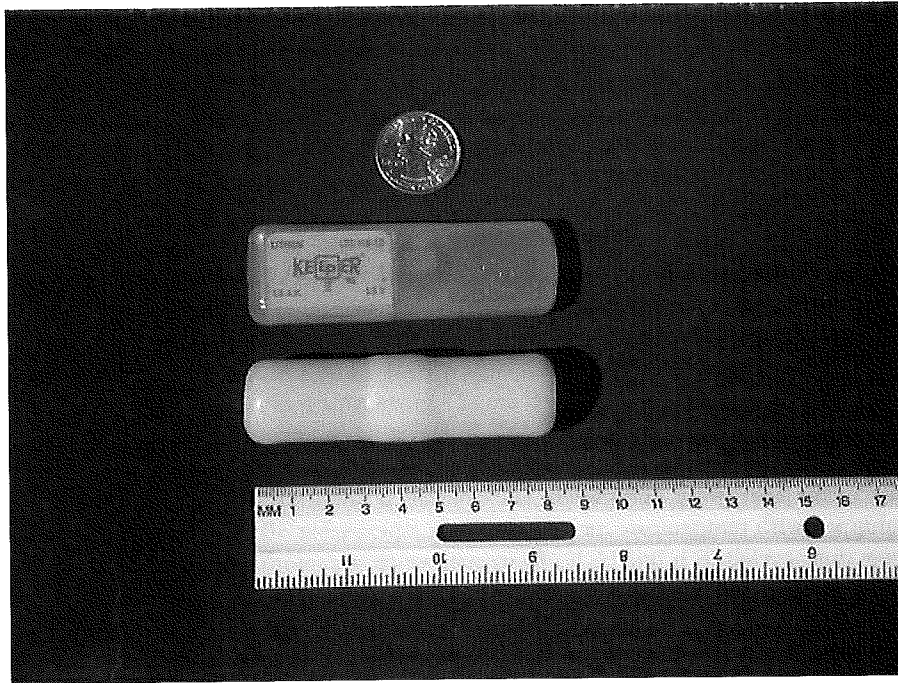
Figure 1. Subcu 16M-3v (top) and IMP/200/L (bottom) transmitters implanted in captive harbor seals during 2000. The IMP/300/L (not shown here) was slightly larger than the IMP/200/L.
