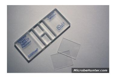
A hemocytometer (or counting chamber) is a specimen slide that is analyzed under a microscope to determine the number of cells in a liquid sample, such as blood.
